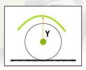
• Based on the above calculation, you would adjust spring preload until you have about 50mm of suspension droop.
