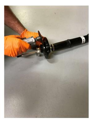
Remove the top locking collar from the Feal shock, slip spring seat over the Feal shock, and reinstall the top locking collar. Make sure the second larger locking collar is 140mm above the center of the eyelet.
