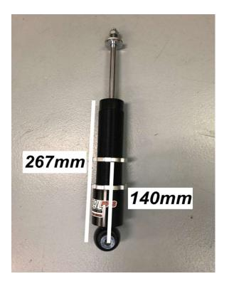
Tighten the top locking collar with provided spanner wrench. Tap the end of the spanner wrench with a hammer to ensure it is tight. Make sure to install the provided washer UNDER the top mount. Reinstall spring and top mount.
